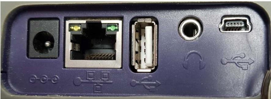
Figure 1: Side panel of Certifier. (Mini-USB on right)
