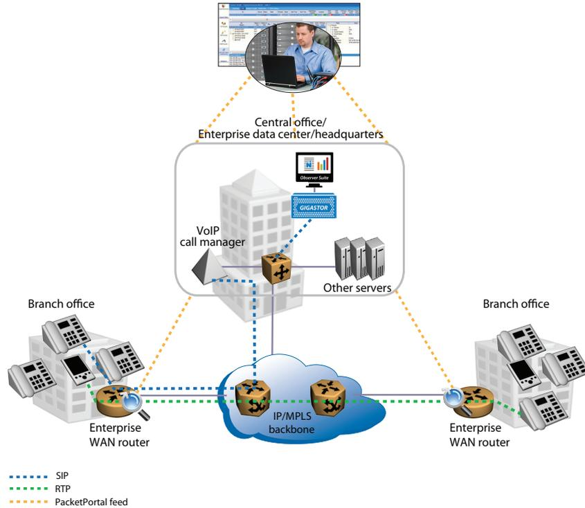
Figure 3. Real-time communications bypass central monitoring
