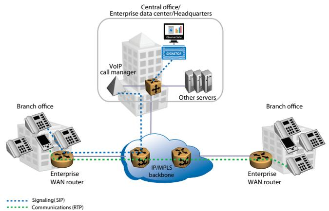
Figure 1. VoIP signal routing and probe location
