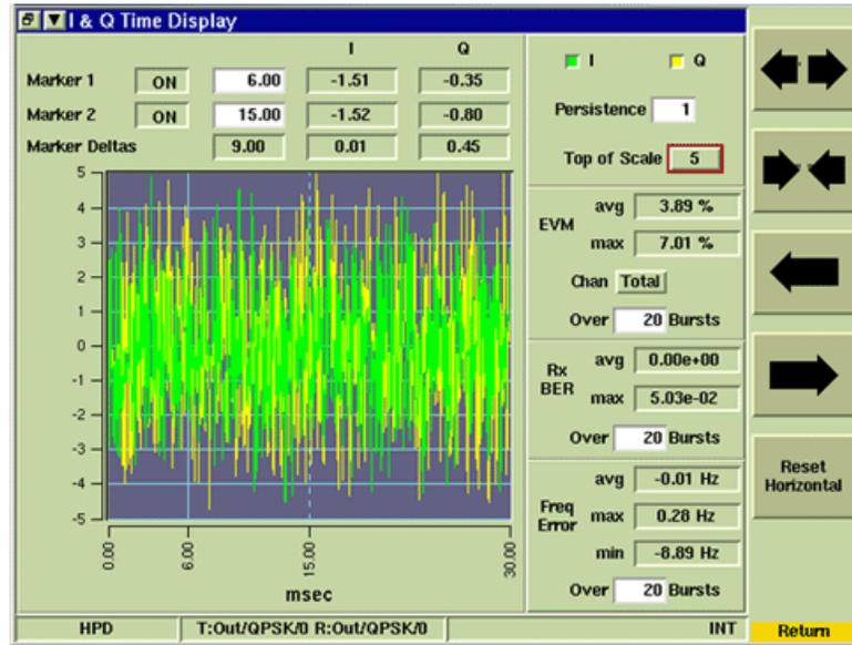
Fig. 3-4 I & Q Display Adjust Horizontal Soft Key Sub-menu
