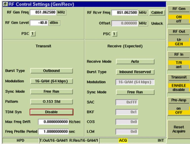
Fig. 6-3 Configure RF Control Settings - MSU Functionality Test
