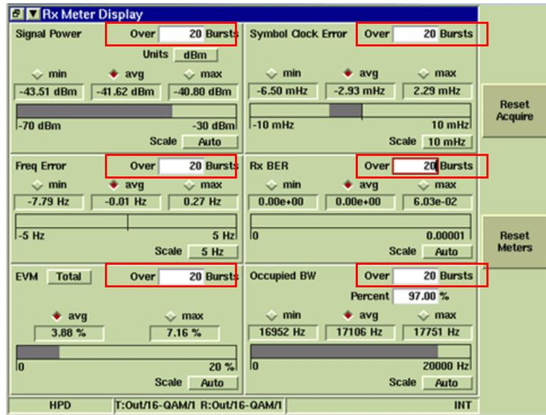
Fig. 6-2 Configure Rx Meter Fields - BR Functionality Test
