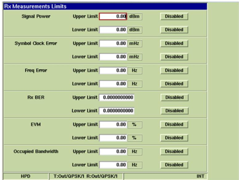
Fig. 2-4 Rx Measurements Configuration Tile
