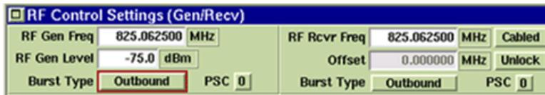
Fig. 2-9 RF Control Settings Tile - Minimized View
