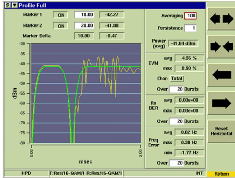
Fig. 3-11 Power Full - First two ms (msec) of Burst
