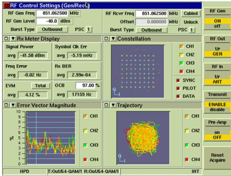
Fig. 5-6 Constellation Tile - 64 QAM Signal
