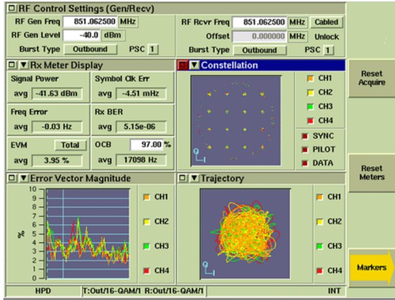
Fig. 5-5 Constellation Tile - 16 QAM Signal
