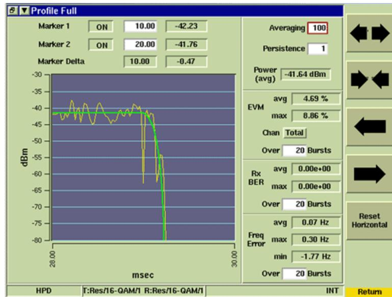
Fig. 3-12 Power Full - Last two ms (msec) of Burst
