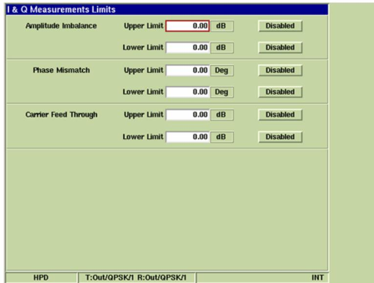
Fig. 2-3 I & Q Measurements Limits Configuration Tile
