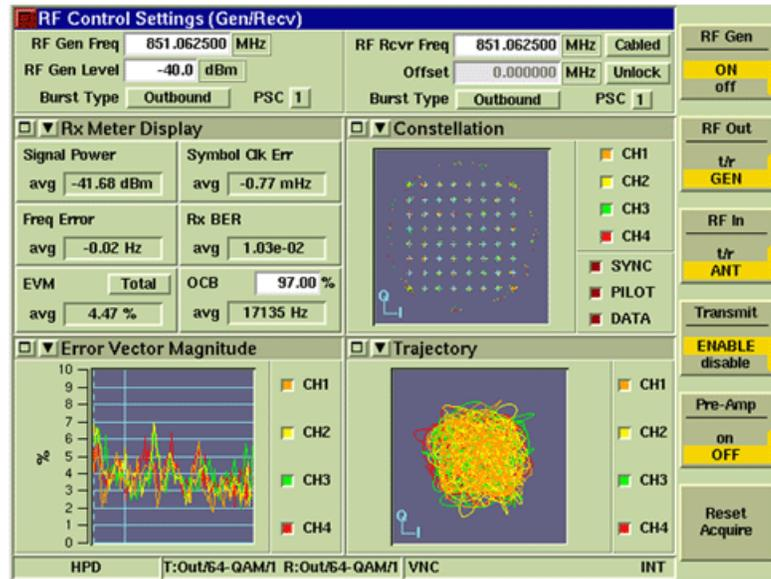
Fig. 5-8 RF Control Settings Tile - Rx BER Measurement
