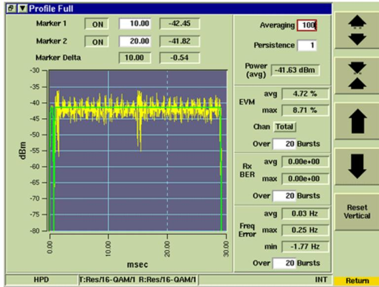
Fig. 3-10 Power Full Adjust Vertical Soft Key Sub-menu
