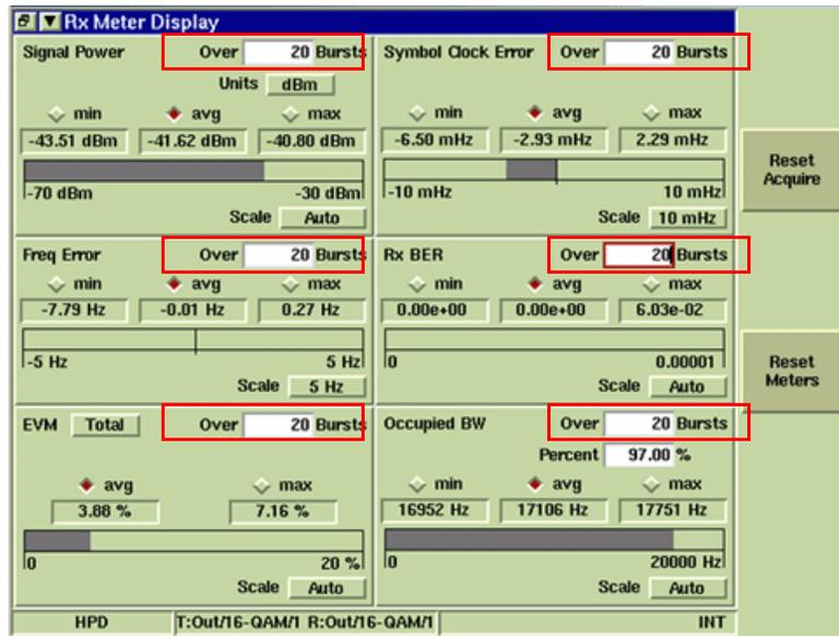
Fig. 6-4 Configure Rx Meter Fields - MSU Functionality Test
