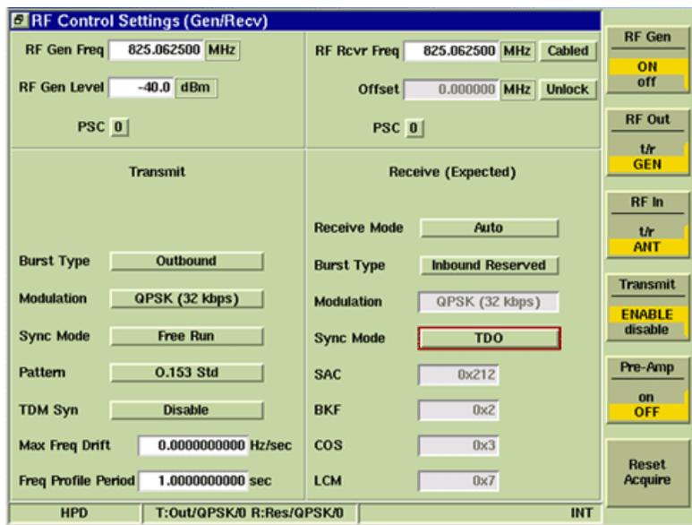
Fig. 2-12 RF Control Settings Tile - TDO (Receive Sync Mode)
