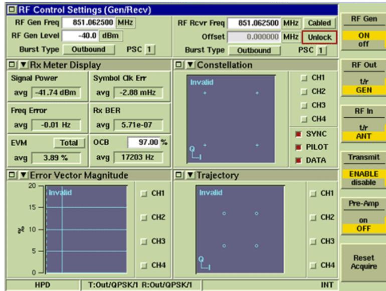
Fig. 5-3 RF Control Settings Soft Keys Enabled
