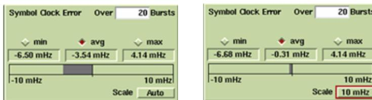
Fig. 2-18 Rx Meter Display - Symbol Clock Error Meter Scale Adjustments
