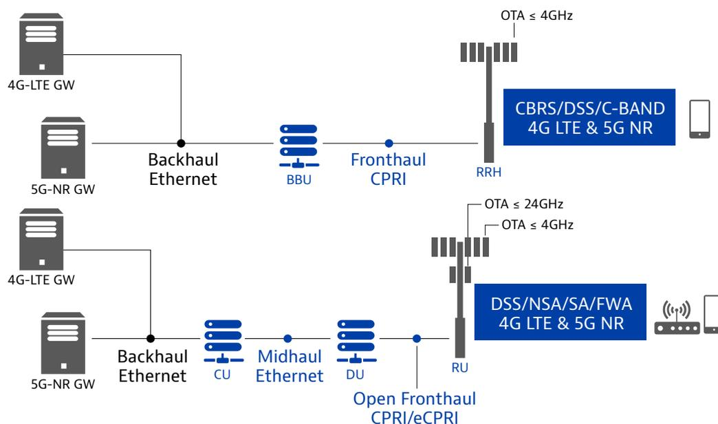
Traditional fronthaul architectures were based on CPRI, where radio elements were designed to receive control signals from the base band unit (BBU) as well as communication of user signals such as downlink and uplink from/to the BBU, respectively. The main function was performing digital/analog conversion and analog signal management for carrier assignment, amplification and filtering.
