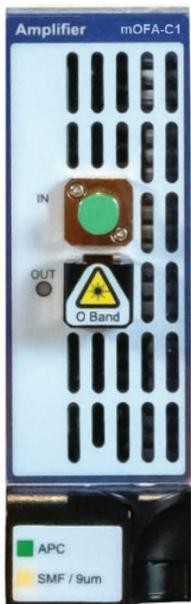
The MAP Optical Fiber Amplifier (mOFA-C1) is the first fiber amplifier optimized for test and measurement applications in the O-band. While simple to control from the front panel or over the remote interface, mOFA-C1 amplifiers meet some of the most demanding optical specifications, including a low noise figure (<6.0 dB) and broad gain across the LAN WDM spectrum.
