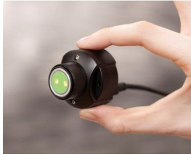
Figure 2: The MicroNIR spectrometer.
