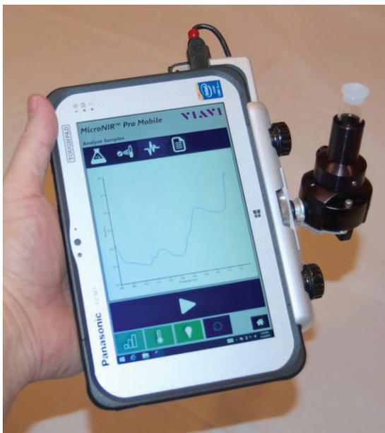
Figure 1. MicroNIR spectrometer tethered to a rugged 7" Windows 8.1 tablet; the MicroNIR is equipped with a vial holder in this image
