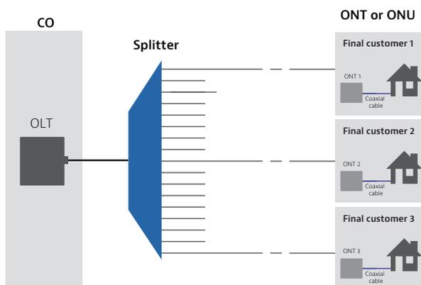
Figure 2. Simple PON Network Topology
