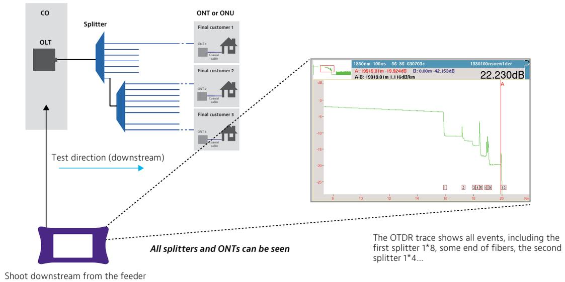
Figure 13. OTDR is Shot Downstream and Trace Displays Many Events that are Difficult to Identify without Exact Network Topology (and corresponding distances)
