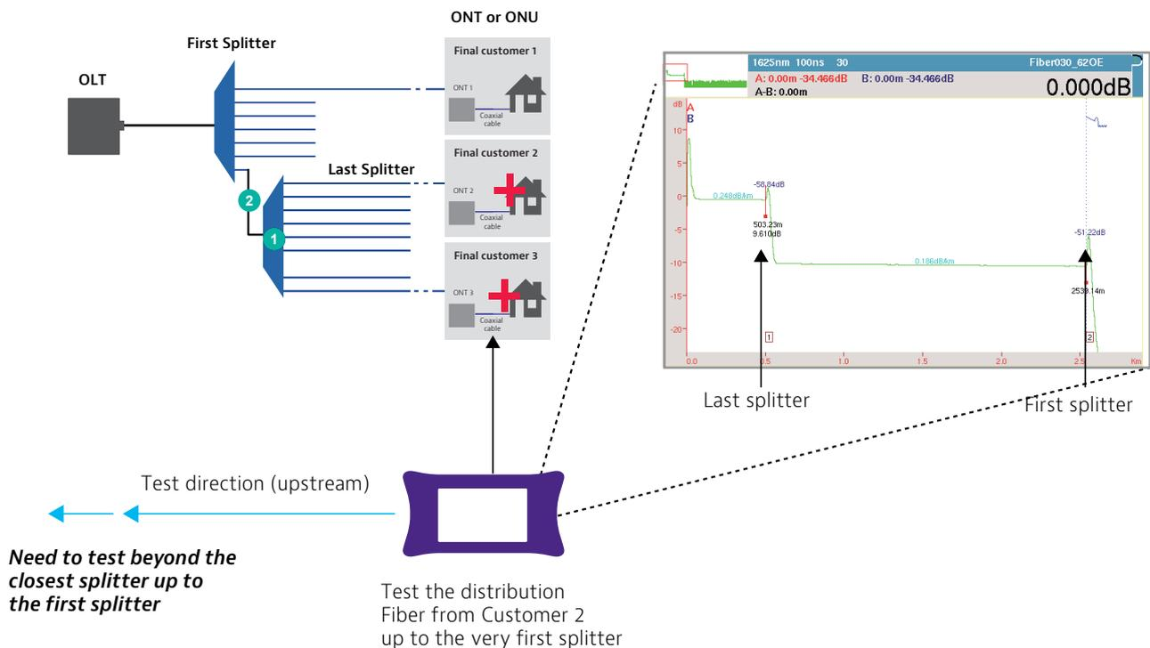
Figure 11. OTDR is Shot Upstream and Trace should Display the Traffic through the Last Splitter up to the First One
