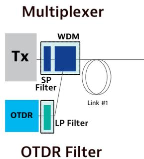
Figure 8. OTDR Insertion for In-service Monitoring
