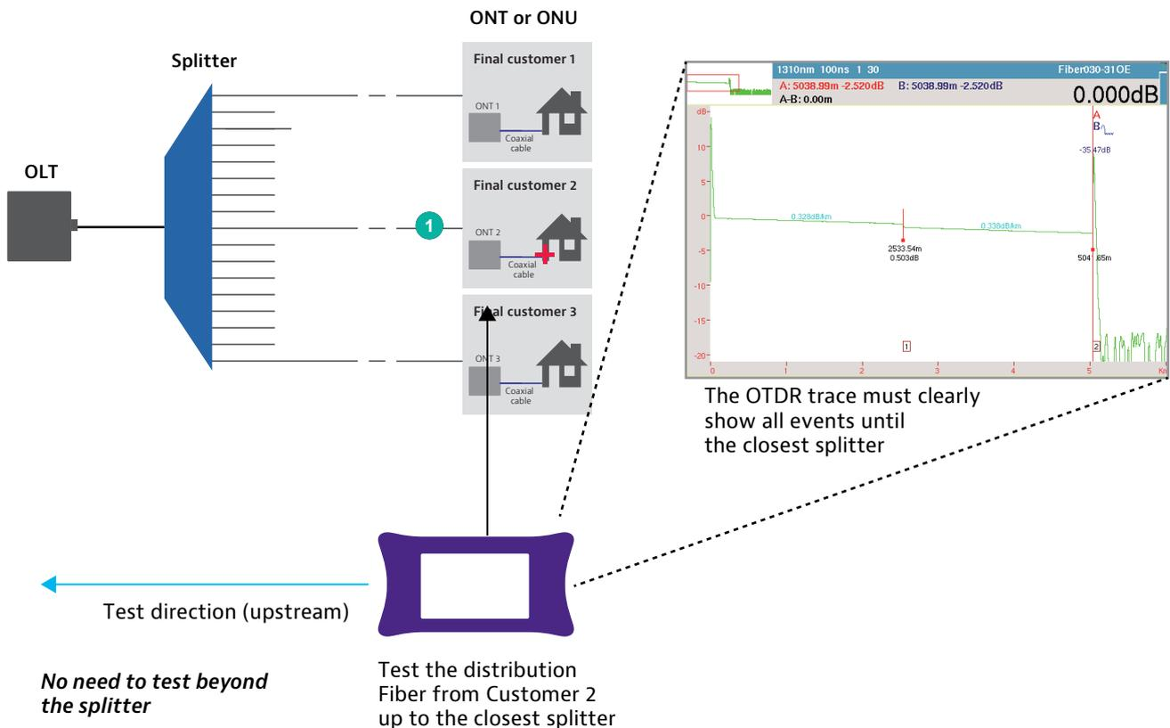
Figure 10. OTDR is Shot Upstream and Trace only Matters up to the Splitter
