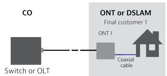
Figure 1. FTTx Case = Point-to-Point FTTx Network
