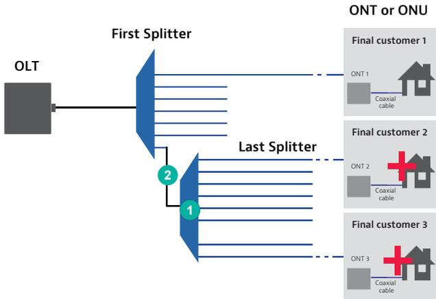
Figure 5. PON Case 2—Cascaded PON with Affected Subscribers Connected to Last Splitter
