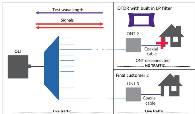
Figure 9. OTDR Insertion for FTTH Troubleshooting at a Customer Location (ONT is disconnected)
