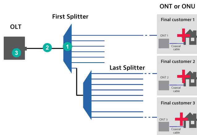
Figure 6. PON Case 3—All Subscribers are Affected (All Connected to the First Splitter)
