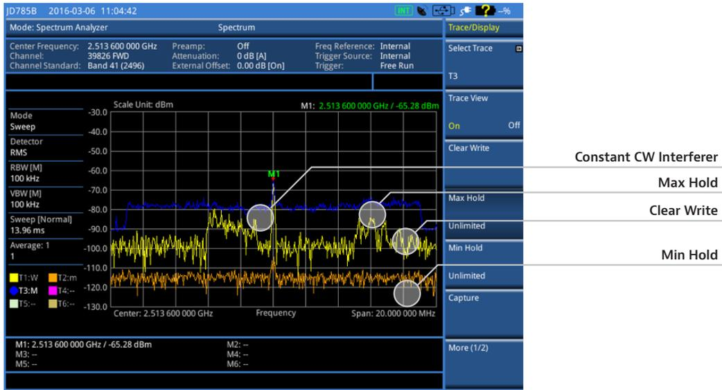
Figure 5. LTE-TDD signal in Spectrum Analyzer mode showing different trace modes
