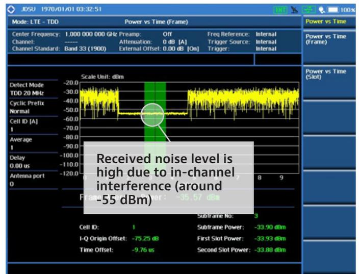
Figure 21b. Power vs. Time (Frame) plot in presence of in-channel interference
