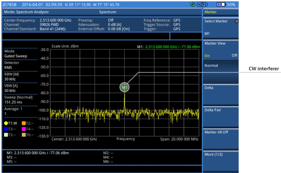
Figure 12. LTE-TDD signal in gated sweep mode, showing CW interference in the uplink
