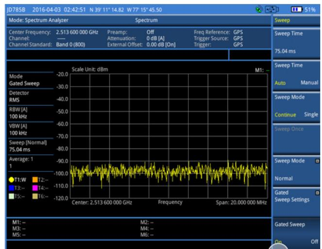
Figure 11b. LTE-TDD spectrum with gated sweep set to on
