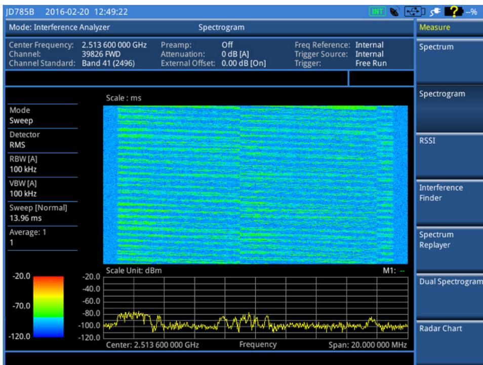
Figure 13. Spectrogram view of a 20 MHz LTE-TDD signal with no interferers (non-gated)
