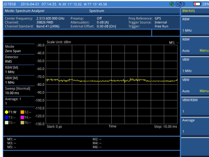
Figure 8. LTE-TDD signal in spectrum analyzer zero span mode in presence of a CW interferer
