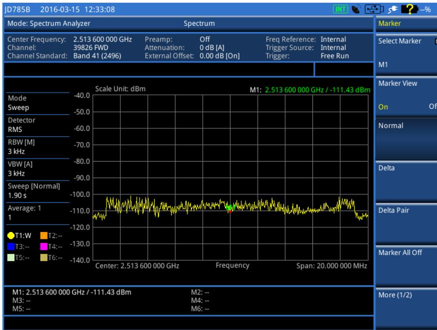
Figure 3. Stable LTE-TDD spectrum
