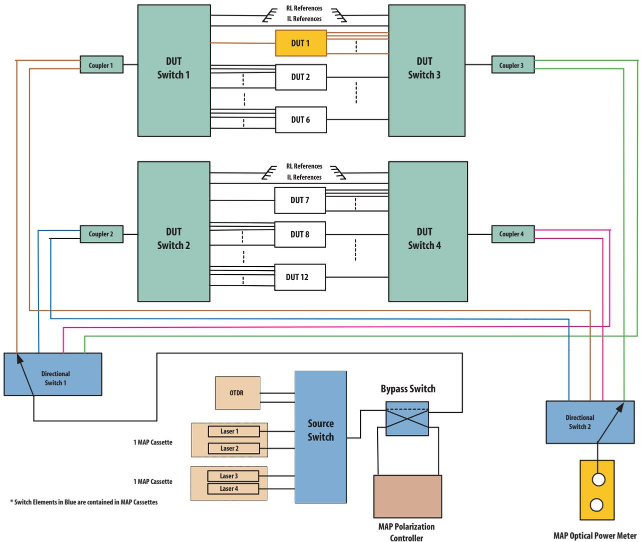
Figure 4: Block diagram of the JDSU OCETplus system, which is capable of executing the 85/85 test and measuring 70 dB RLs.
