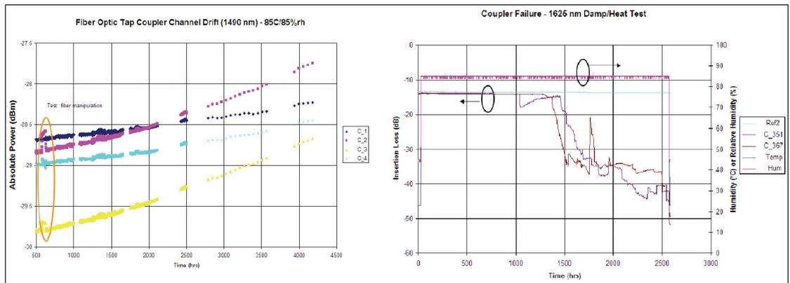
Figure 9: Test to failure examples. The first device shows a slow continuous change in loss where the second device fails catastrophically
