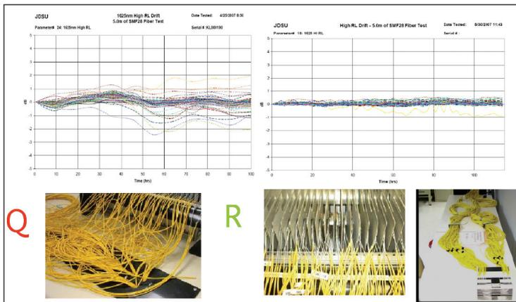
Figure 7: Bad fiber management can lead to poor system performance. Micro bends can cause IL that can change over time as the fiber relaxes.
