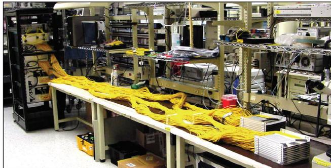
Figure 6: A JDSU OCETplus system is prepared for baseline referencing. The 5 m pigtailed from the DUT switches are spliced together. Splices are managed on trays with strain relief holders.
