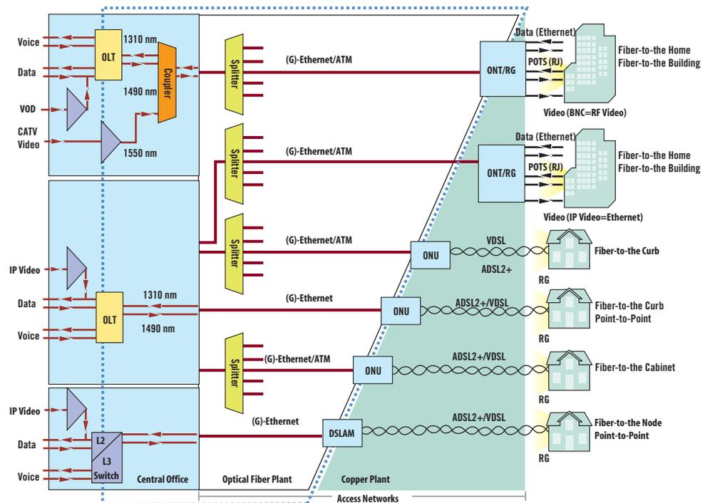
Figure 1: Typical FTTx architectures. The optical layer components are contained within the blue hashed box
