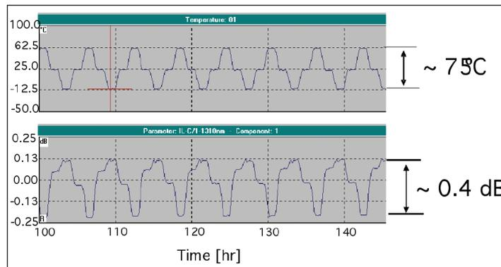
Figure 8: The shape and stability of the IL changes over temperature cycling can give the designer guidance on improvements to make.
