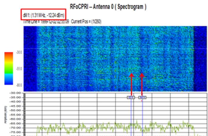
Comparative spectrogram results showing consistent interference on both antennas; note rolling rises in the noise floor across the whole band
