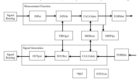
All SCPI commands are based on a hierarchical tree structure consisting of keywords and parameters. Associated commands are grouped together under a common node in the hierarchy.
