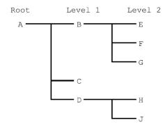
All SCPI commands are terminated by a line feed (0x0A). After termination the pointer is returned to the root.
