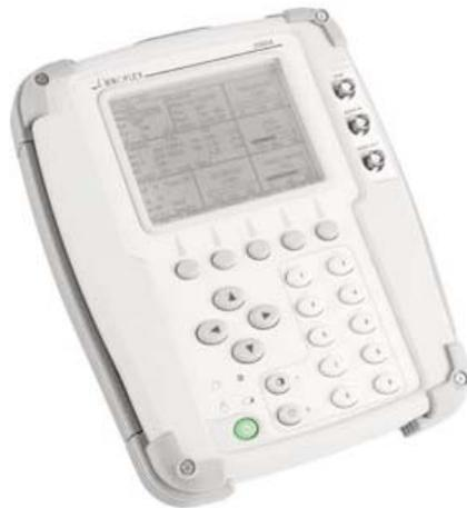
The 3500A Radio Test Set was developed to be able to quickly test and verify the operation of complete radio systems. A complete verification of a radio system includes testing of the transmitter and receiver of the radio as well as the duplexers, cables and antennas.
