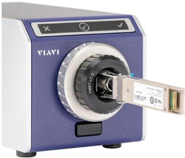
Technicians can leverage the FVAM-2000's built-in intelligence to streamline the fiber inspection process. By automating setup, tip configuration, testing, and data storage, it replaces the need for outdated manual devices. Simply attach the desired adapter and let the microscope handle the rest:
