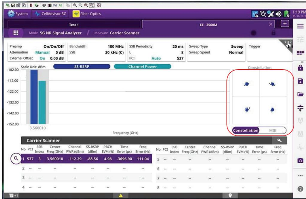
Figure 11. The CA5G QPSK constellation plot of SSB
