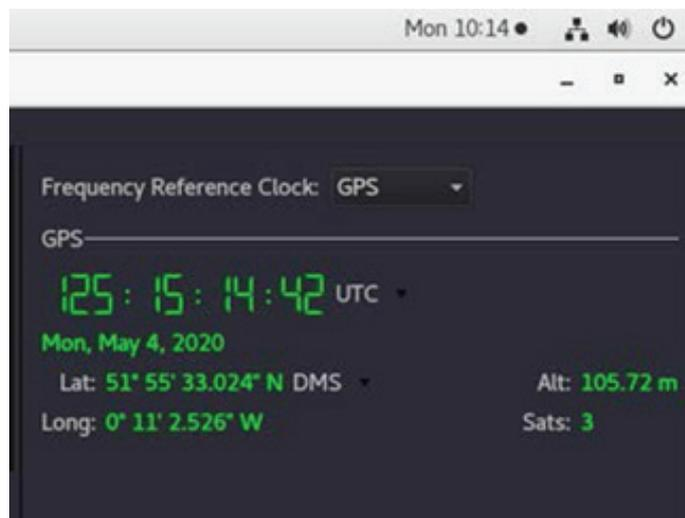
Figure 2. The Ranger's GNSS receiver information (example)
