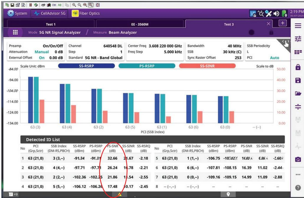
Figure 8. The CA5G Beam Analyzer '3' Network SCR Analysis
