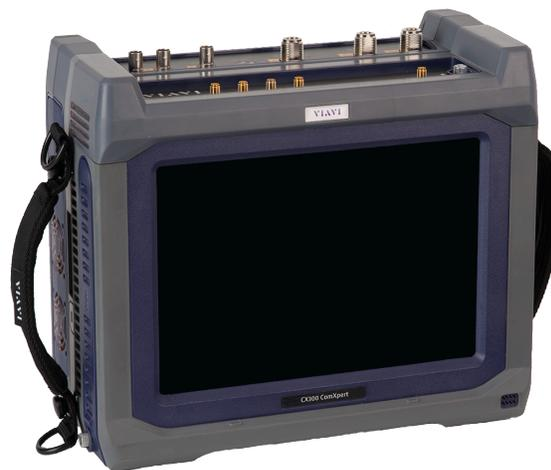
Figure 1-1 CX300 ComXpert Communications Service Monitor
