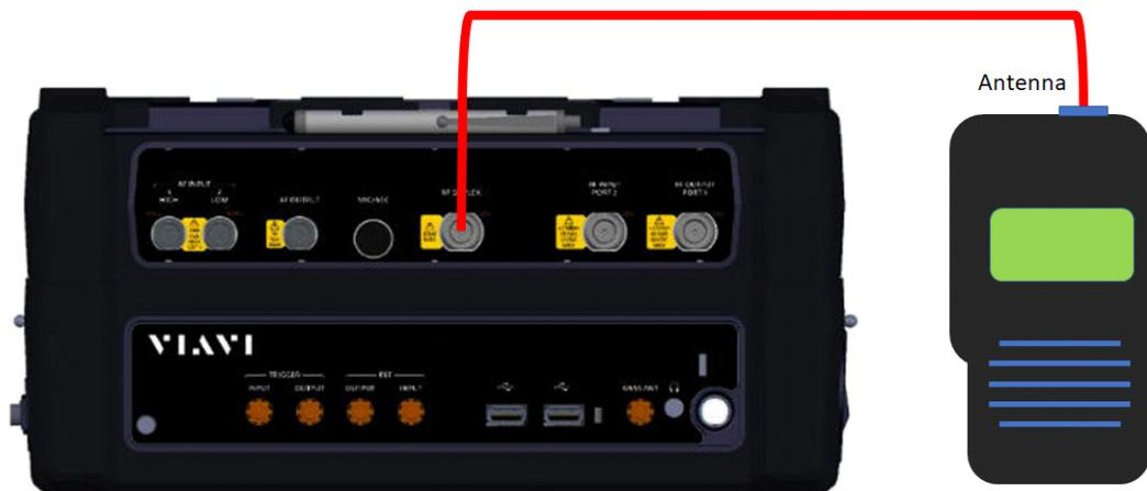
Figure 3-1 DMR Transceiver Test Setup Diagram
