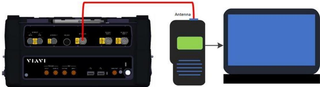
Figure 3-2 DMR Receiver Sensitivity Test Setup Diagram
