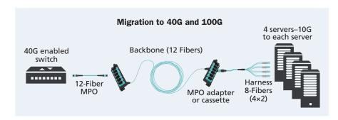
Migrating to 40/100G requires the initial step of changing one end to connect to equipment by connecting an MPO equipment cord to a QSFP port. This eliminates the cassette and duplex cords, or the harnesses.
