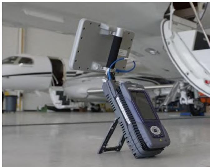
**Figure 3-2 Over-the-Air Test Set-Up**
