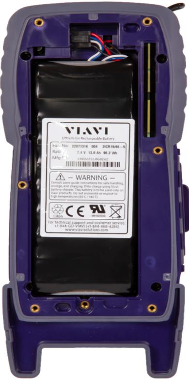
Figure F-4 Replacement Battery / Location
