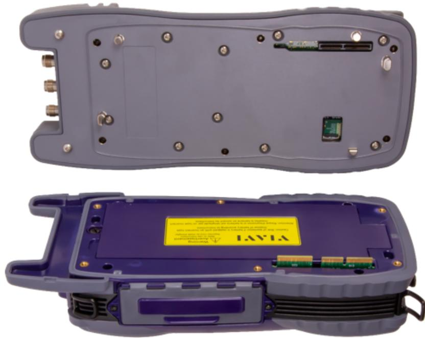
**Figure 12-3 Battery Cover Removal**
