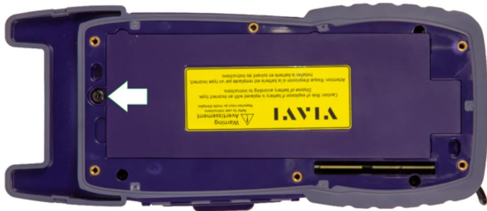
**Figure 12-4 Battery Cover Screw Removal**
