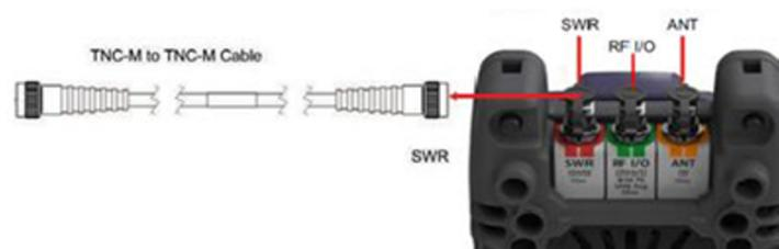
Figure 10-2 VSWR Calibration RF Port Setup
