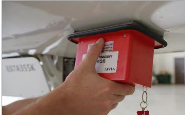
**Figure 3-1 Coupler Test Setup**
