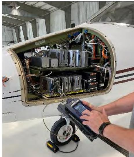
**Figure 3-5 Direct to UUT Test Setup**
