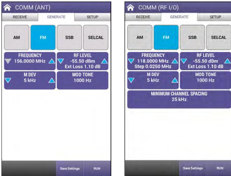
Figure 7-8 VHF COMM Frequency Modulation (FM) Generate
