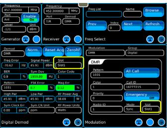
The receiver RX Sensitivity can be measured by lowering the RF Generator level until an indication near 1% BER is indicated. This is the approximate sensitivity of the receiver portion of the repeater.
