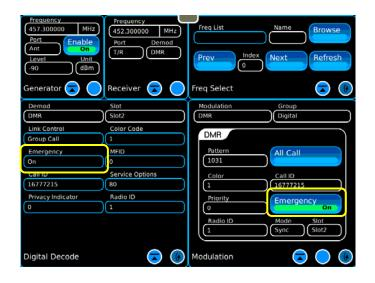
The Emergency feature can be tested by enabling the emergency button on the Generator Modulator Tile and monitoring the Digital Decode emergency field.
