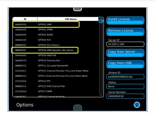
Option 06 must be enabled to use the DMR Repeater Test function.
