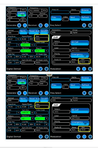
Select the Enable button on the Generator Tile and the repeater should begin to transmit.
