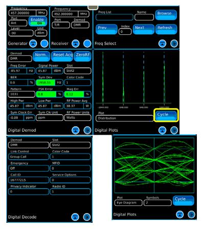
Select the Fast Stack Icon on the Modulator Tile to reveal the Digital Plots Tile.
