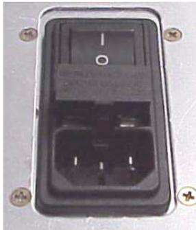
5. Remove Fuse Carrier from Test Set.
