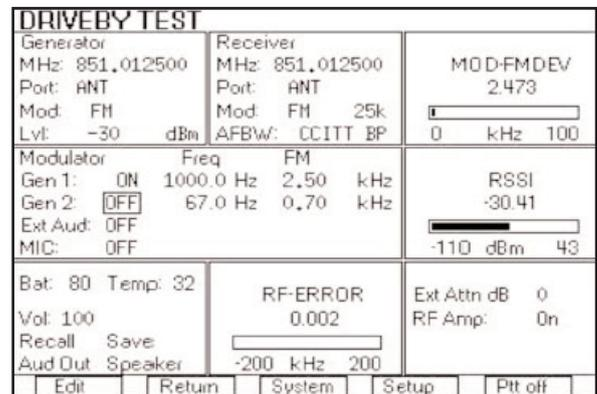
*Figure 3.0 The 3500 over the air test screen*
