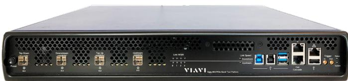
The Xgig® 4K4 platform provides protocol analysis for PCIe 4th generation traffic at all layers of the stack. It supports link widths up to 4-lanes, and link speeds to 16GTps.
