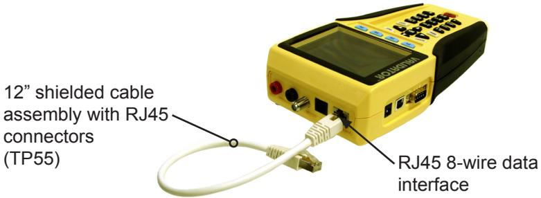
12" shielded cable assembly with RJ45 connectors (TP55)
