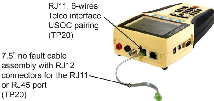
RJ11, 6-wires Telco interface USOC pairing (TP20)
