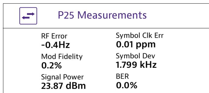
Figure 1.0 - Modulation Fidelity Measurements
