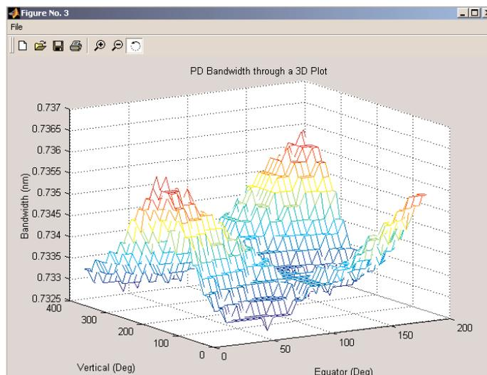
Figure 9. The polarization dependent BW across the Poincare sphere
