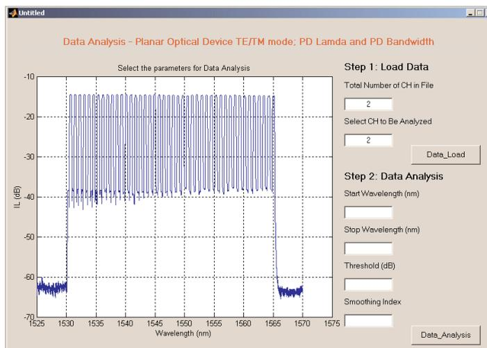
Figure 10. GUI for TE/TM loss application
