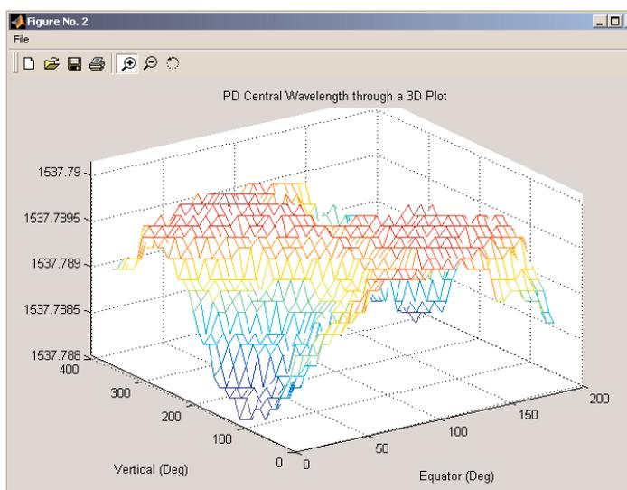
Figure 15. The polarization dependent CW across the Poincare sphere
