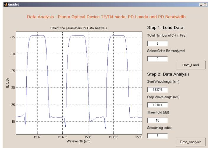
Figure 11. Zoom the analyzed area and input the data analysis parameters
