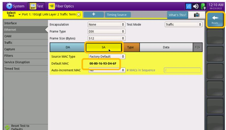
Figure 12: Ethernet Setup, Source MAC
