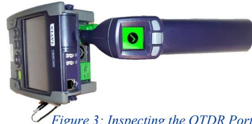
Figure 3: Inspecting the OTDR Port
