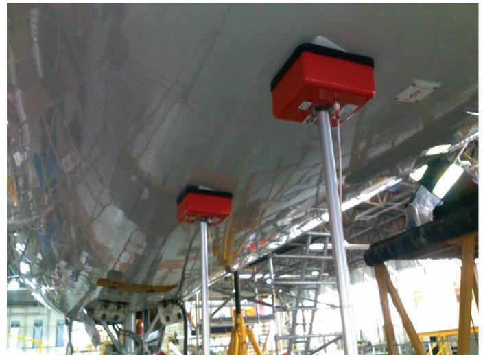
Non-intrusive testing method using supplied couplers simulates flight conditions
