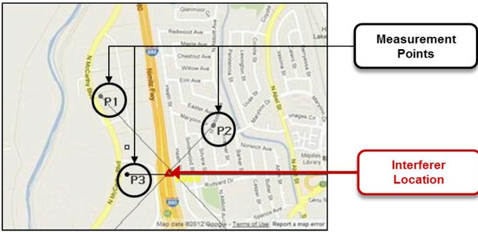
Fig 16. Triangulating the Interferer
