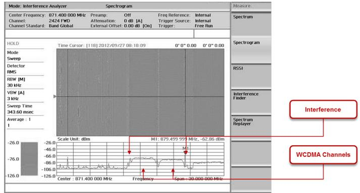
Fig 12. Detecting Intermittent Interference Signals
