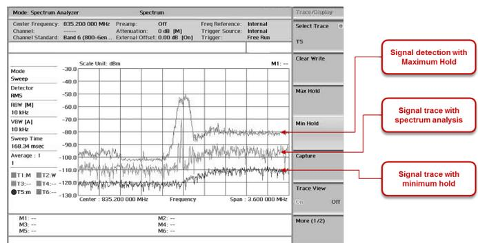
Fig. 6 Detecting intermittent signals with maximum power hold
