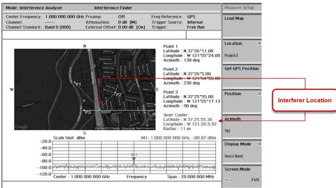
Fig 17. Interference Location
