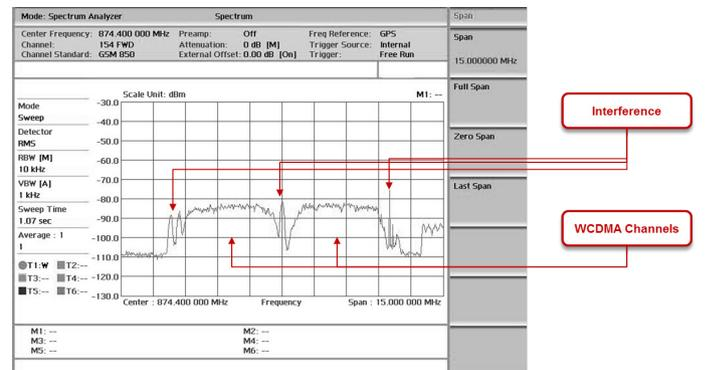
Fig 13. WCDMA Channels with Interference
