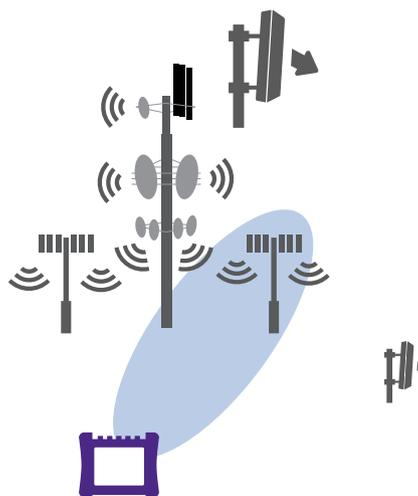
Fig 15. Interference Location with Directional Antenna
