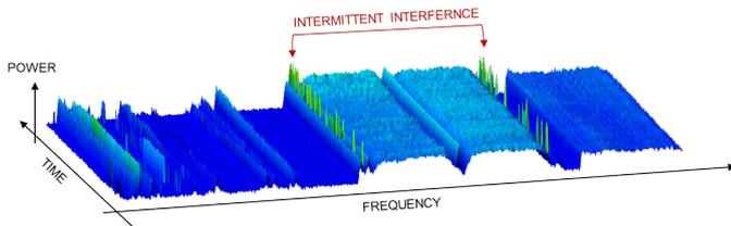
Fig 11. Intermittent Interference
