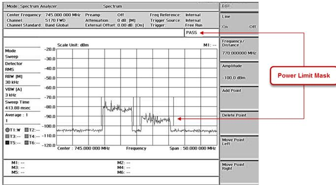
Fig 10. Spectrum Clearance Mask
