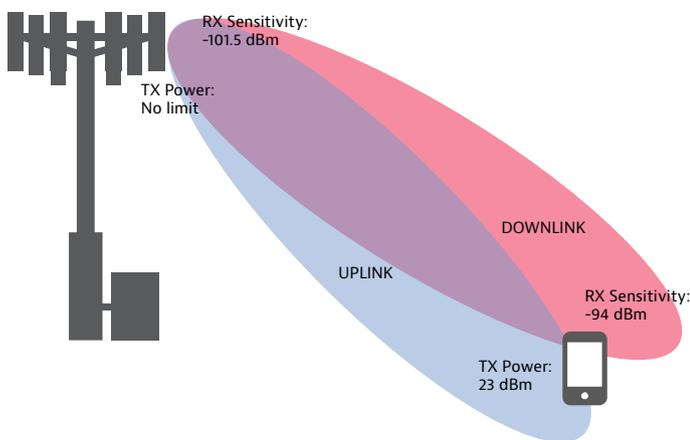
Fig 2. LTE-TDD (10 MHz) Transmission and Sensitivity Requirements
