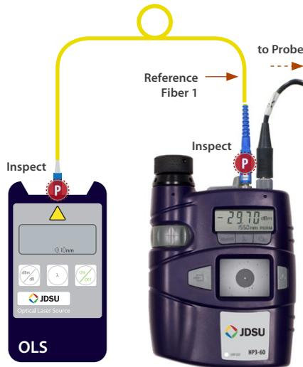
1. **Inspect**, and if necessary, **clean** both ends of **reference fiber 1**.
