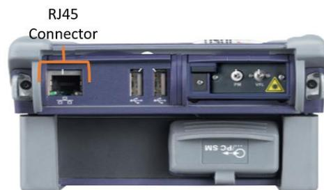
Figure 5: T-BERD/MTS 2000, Top view
