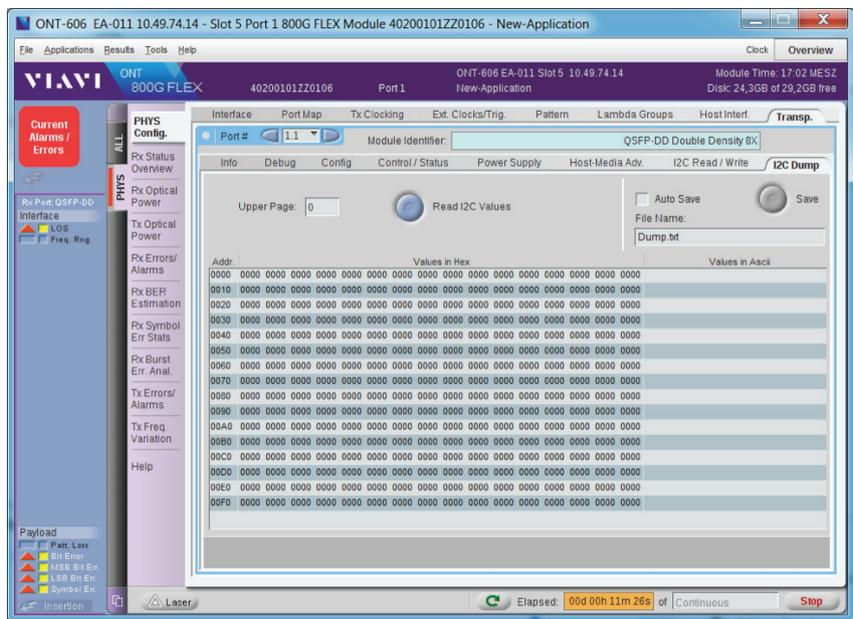
The above screen shows the memory dump of the first page of memory. This can quickly check if the correct values have been stored in the QSFP-DD EEPROM. Blank or random data may indicate a device has not yet been initialized.
