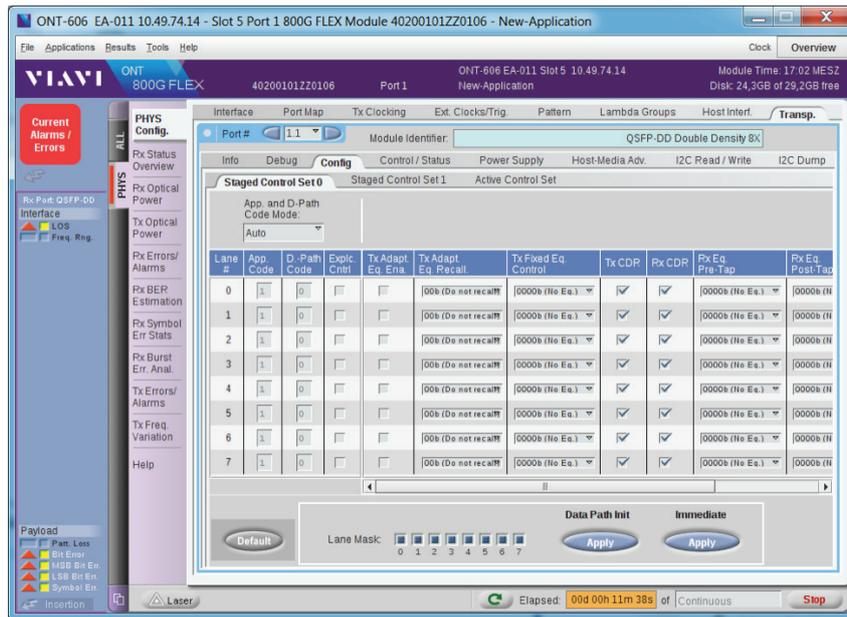
Some of the more advanced applications in the module management application allow precise and exact control of the module electrical parameters in a clear and unambiguous manner.
