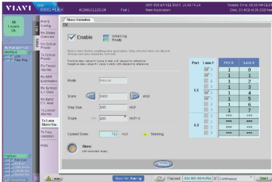
The above screen shot shows the dynamic skew application for PAM-4. The ability to precisely control the relative timing of transmitted lanes to a fraction of a UI and still retain 'hitless' phase shifting is key to resolving challenging problems including crosstalk and DSP based firmware timing issues.
