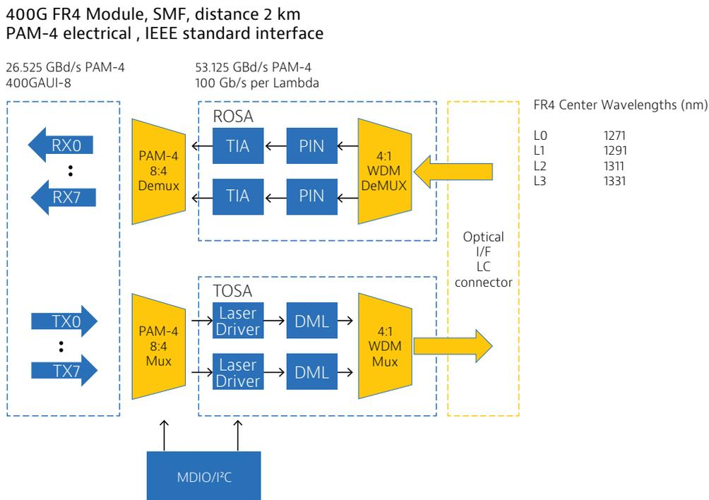
The FR4 interface will also have widespread applications, including with telcos. It offers a longer link budget of 2 km over one single mode fiber. The 400G is carried on four 100G signals, each on a slightly different wavelength.
