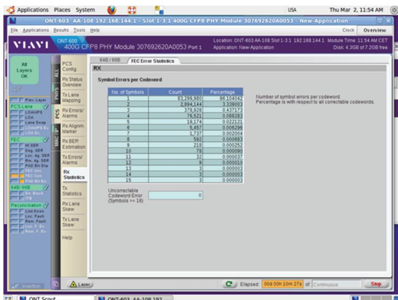
The screen shot below shows the case where a serious issue is occurring. Although the FEC has significant margin (we see a maximum of 4 error symbols in a codeword) the distribution is not monotonic and shows that this system has an underlying error source at work. Note that this example for a 100G link was generated by a special VIAVI ONT application which can create a wide range of FEC error distributions to stress and validate FEC logic and power integrity.
