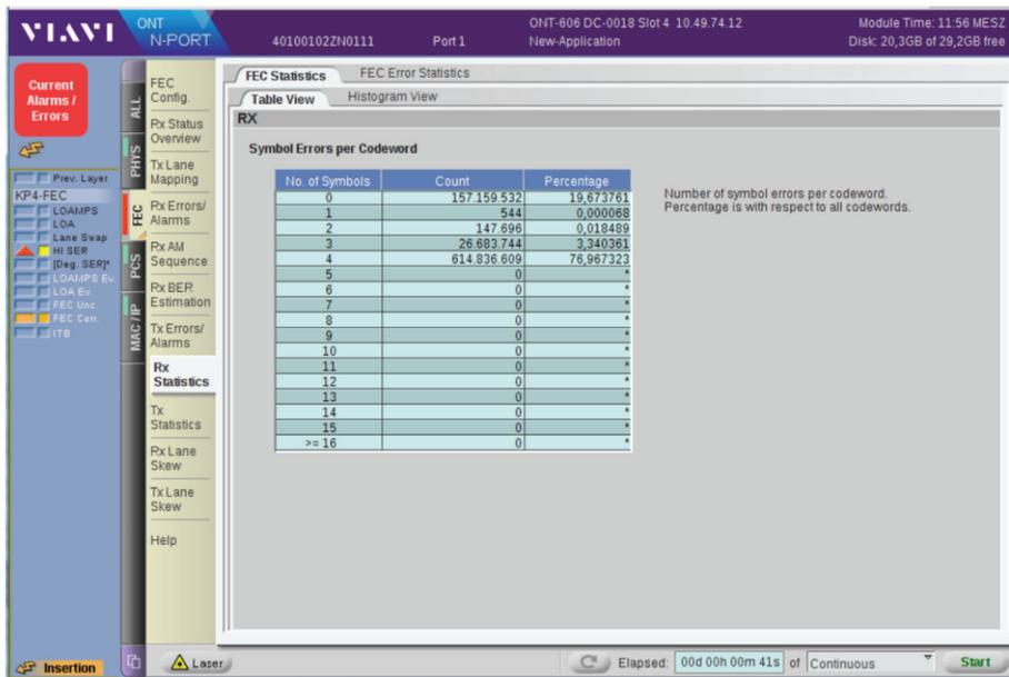
The ONT has the ability to both analyze error distributions and patterns across a whole sequence and track the error profile on a per PAM-4 symbol basis.
