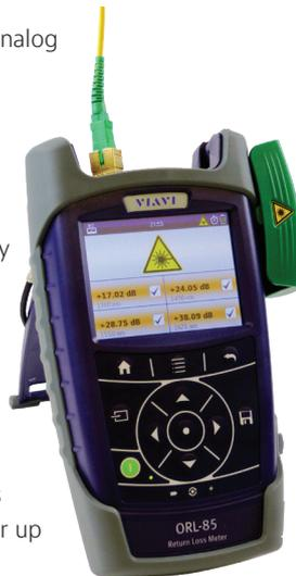
The ORL-85 is compatible with the P5000i digital analysis microscope for checking fiber end-face quality and getting pass/fail acceptance results at the push of a button.
