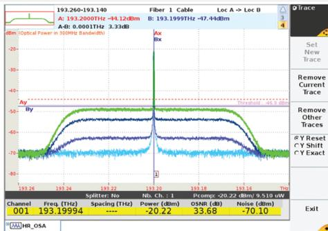
Varying power levels of OSNR inside a DWDM channel
