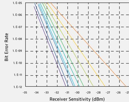
BER measured as a function of power delivered to the RX
