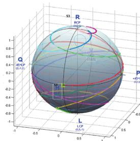
Emulate changes to the state of the polarization as it interacts with small changes in the optical fiber
