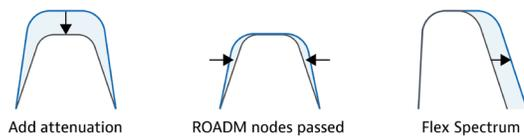
Emulates the DWDM Network Filter & ensures only In-Band OSNR reaches the RX
