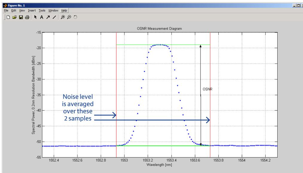
Figure 5. OSNR measurement method (Note that  $\sim 3 \text{ dB}$  must be removed from the NL to convert the measurement 0.2 nm integration bandwidth to the conventional 0.1 nm)
