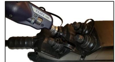
Figure 11: OptiTap Bulkhead
