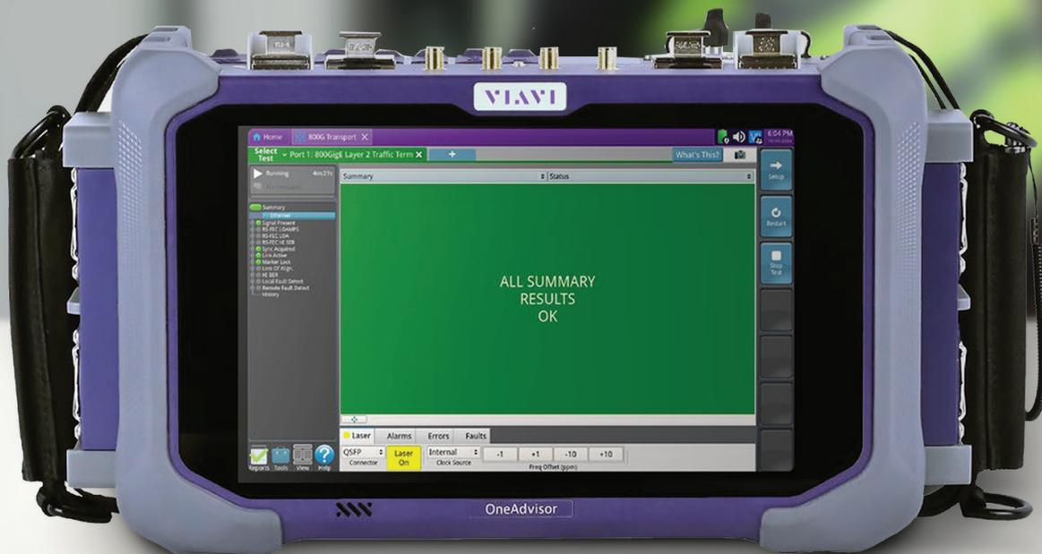
The OneAdvisor 800 delivers all the test capabilities technicians and engineers need to install and maintain high-capacity networks up to 800G. Its portability and modularity make OneAdvisor 800 perfectly suited for metro/core, data center interconnect, and business services testing. The OneAdvisor 800 800G Transport Module supports testing up to 800GE and features the same user interface as all in the T-BERD/MTS Family.
