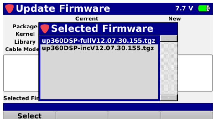
5. Once the file has been transferred from the USB flash drive, the new firmware information will be displayed as shown in the image to the right. Select the **Install** softkey to install the firmware file.
