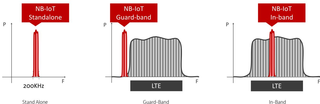
NB-IoT in coexistence with LTE can operate in the following bands:
