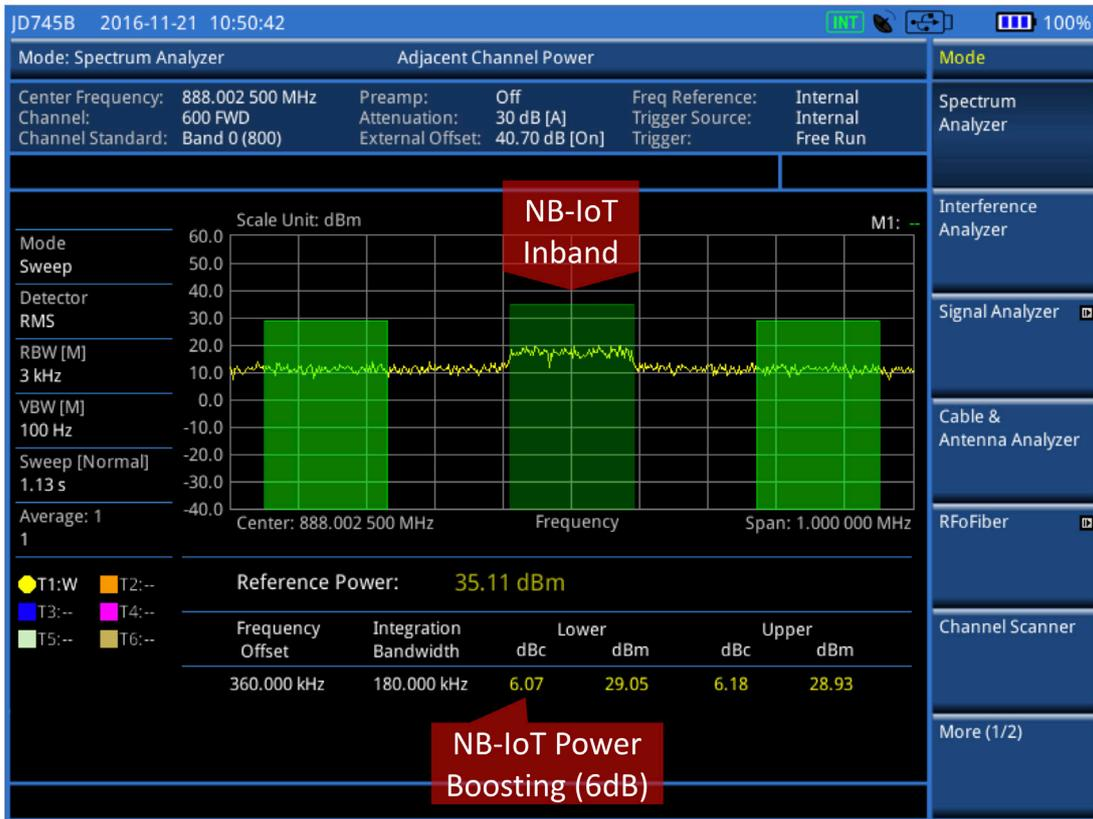
CellAdvisor NB-IoT Adjacent Channel Power Test and Power Boosting Verification
