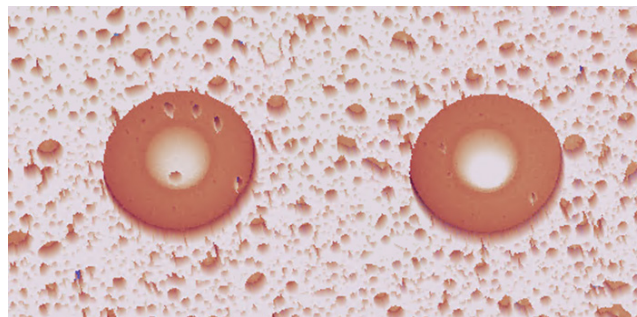
Figure 5. 3D view of a dual fiber using the mFVU
