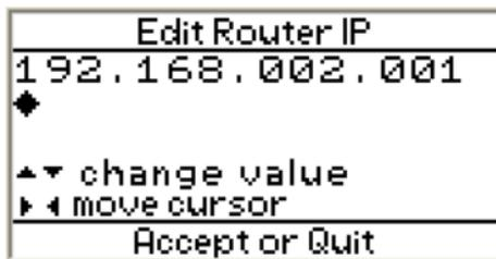
**Figure 11** The Edit Router IP screen
