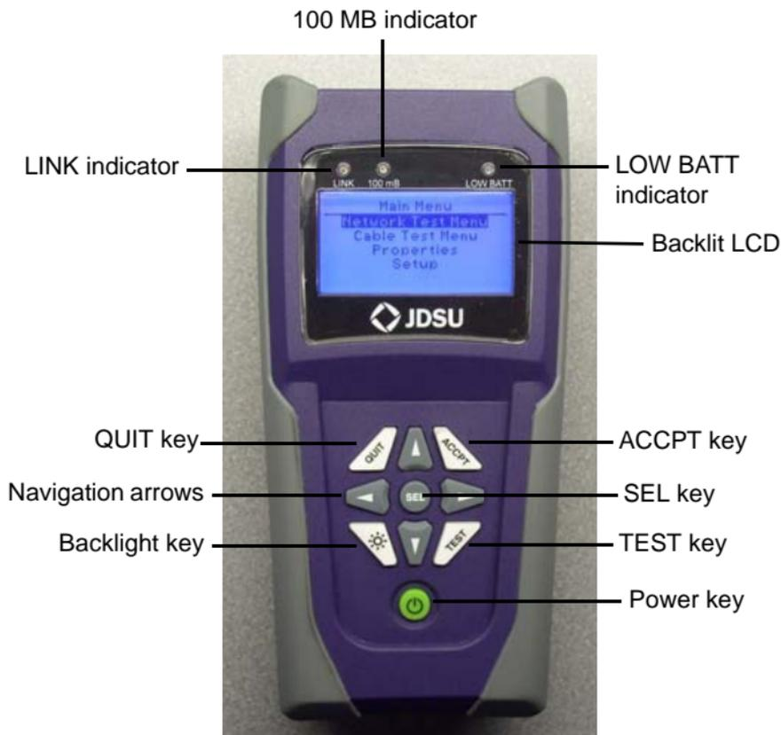
**Figure 2** LanScaperPRO front panel
