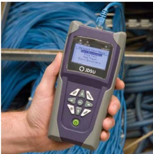
**Figure 1** The LanScaperPRO Network Tester
