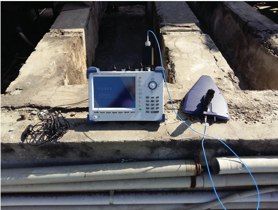
Figure 4: AntennaAdvisor used to identify interference source
