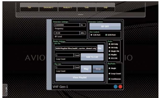
To monitor the multi-carrier waveform, connect the ATB-7300 GEN port to the ANT port. From the Analyzer-1 dropdown menu, select VHF-1. Select the Spectrum tab, set Port Control: to ANT Port and set the following inputs.
