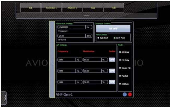
Set the Generator Frequency to 126 MHz, RF Level to -20 dBm, Port Control to GEN Port, and turn the RF ON.
