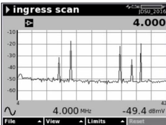
1 - Swept Spectrum Analyzer showing spikes where Cable modem traffic is present since it can only measure energy at frequencies it is currently turned to
