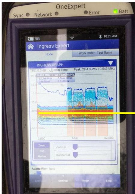
The yellow line is at about -30dBmV on the display. A higher a noise floor than previously seen at directional test points off the active devices.
