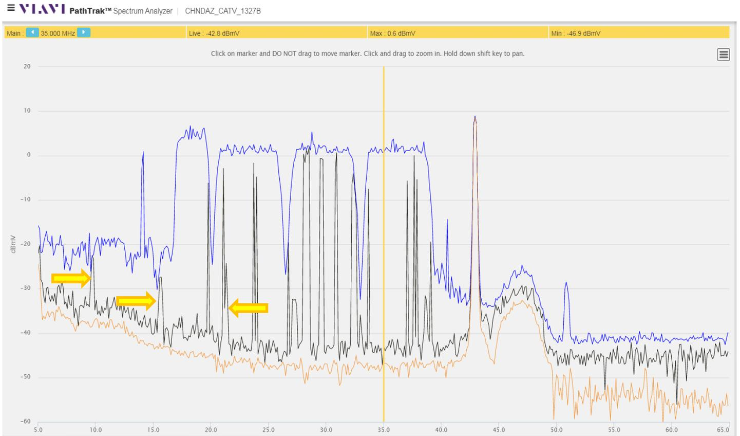
3. Using PathTrak the techs determined the presence of CPD, showing up as lower level spikes (examples of the CPD are pointed out by the yellow arrows above)
