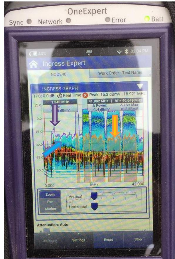
6. Toggled several of the traces On / Off while at this node to determine which ones may help the most with this type of intermittent noise source. It was determined the Live Max, Noise, Heatmap, and Power traces when enabled appeared to best show this noise was present.
