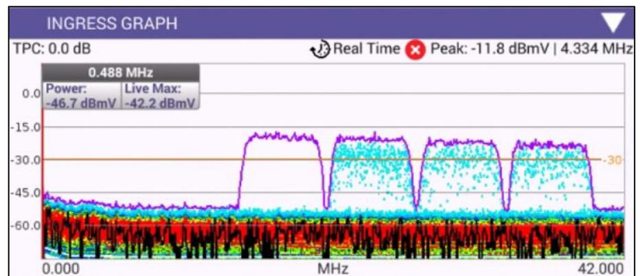
2 - Real-Time Analyzer showing all signals at all frequencies, clearly shows the outline of 4 active upstream QAM channels. Note the difference in view of the same signal between the real-time (above) vs swept spectrum analyzer (Left).
