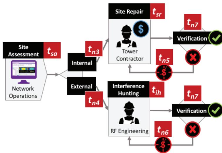
Maintenance process with CPRIAdvisor for interference
