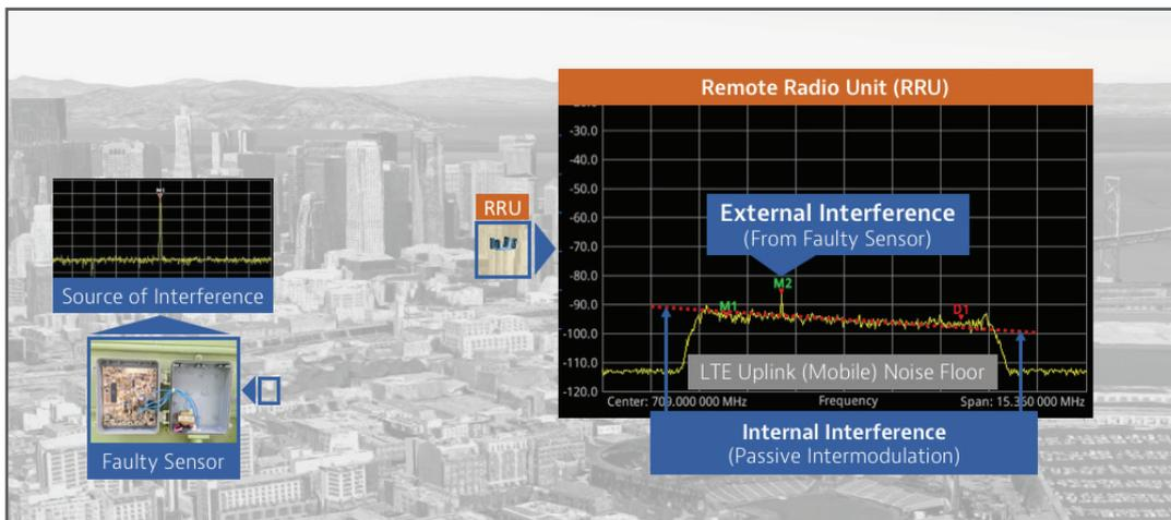
External interference from AC controller and internal interference from PIM
