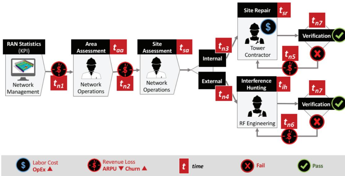
Conventional maintenance process for interference
