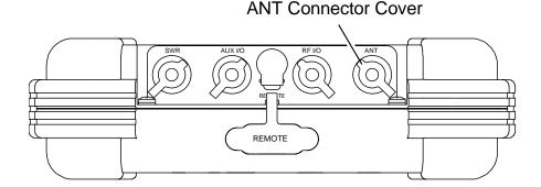
2) Connect High Efficiency Antenna to IFR4000 ANT Connector.
