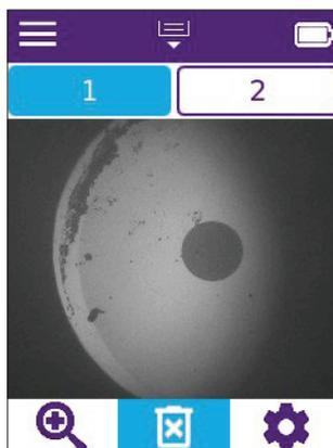
**Step 5.** Short press the trigger to capture an image of the fiber end face. The LED ring lights purple. If the microscope speaker is ON, the sound of a camera shutter is emitted.
