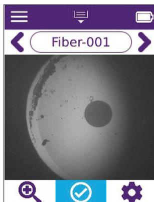
**Step 4.** Short press the microscope trigger to display the **Test Navigation** bar on the **Home** screen. The live image on the **Home** screen indicates that position 1 is selected.
