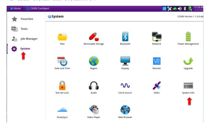
3. Insert a USB stick into one of the USB slots. In the "SYSTEM INFO" screen, SELECT "COPY SYSTEM INFO TO FILE"
