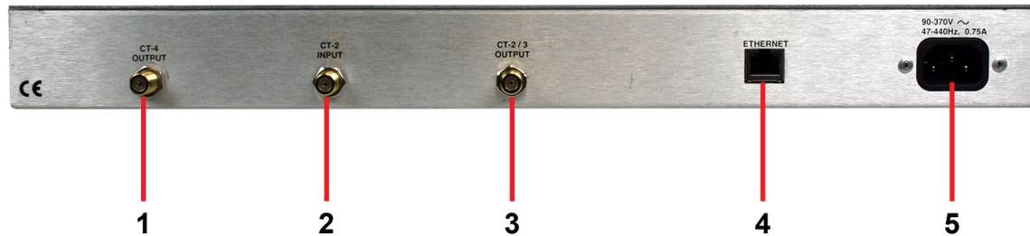
1. **CT-4 Output** – This is the RF output connection for the CT-4 function.
